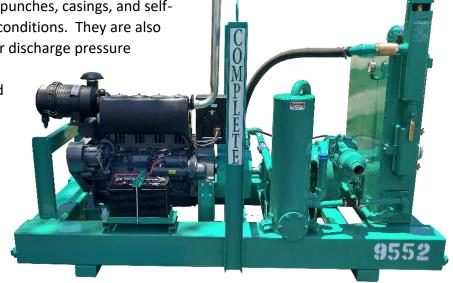
Standard model (2-1/2 VAJP) for hand jetting and small punches or casings. High pressure model (3 VAJP) for large punches or casings or hose runs greater than 400'.
